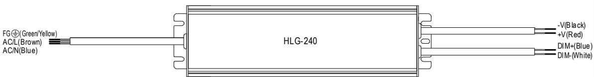
※ Built-in 3 in 1 dimming function, IP67 rated. Output constant current level can be adjusted through output cable by connecting a resistance or 1 ~ 10Vdc or 10V PWM signal between DIM+ and DIM-.
