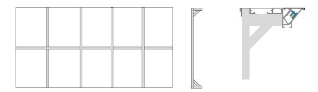
Support frame out of square profiles (e.g., 40x20x3) in a horizontal and vertical pitch of 80 to 100 cm
